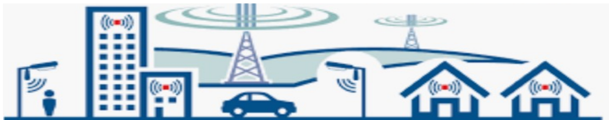
5G combines long and short range antennas connected to the internet via fiber optic cable,
